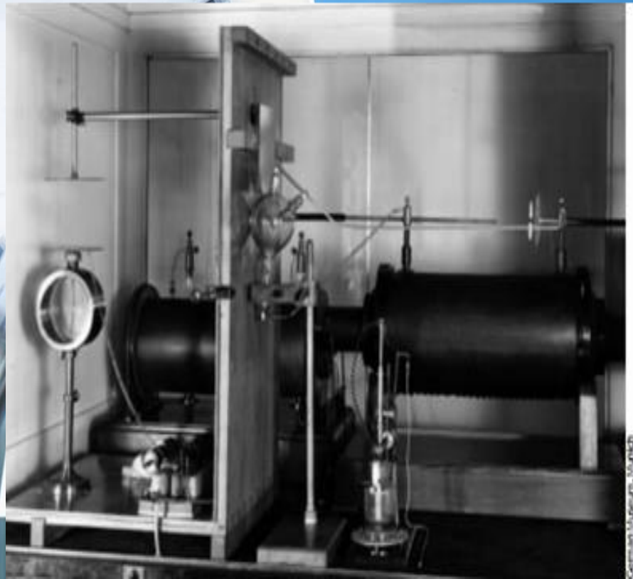
Roentgen's apparatus for studying the ionization of air by X rays, 1906.
